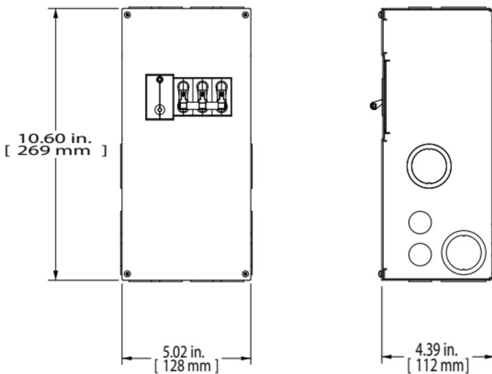
Figure 1. GFPD-150V Box Dimensions
