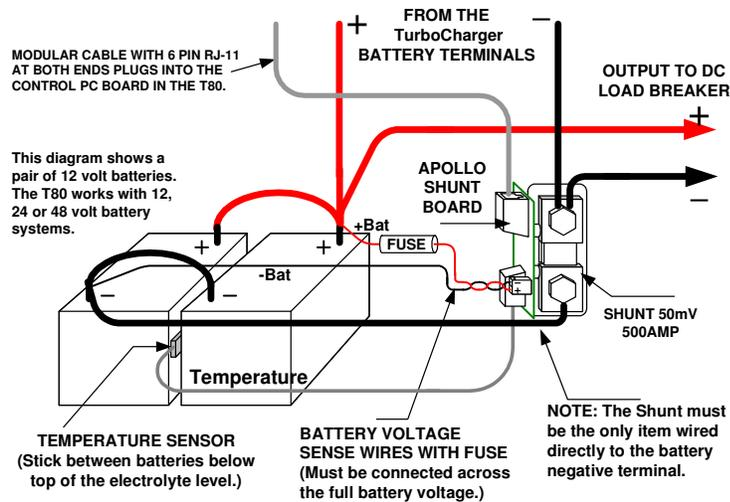
Voltage Sense Wire Installation— Push the white connector on the wire assembly onto the white connector on the Apollo Shunt circuit board after connecting the red wire to a battery positive buss and the black wire to a battery negative buss within the DC load center. Be sure to observe correct polarity when installing voltage sense wires or damage will result. Note: Fuse on positive battery terminal (1/2A 5mm x 20mm fuse).
