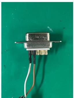
①①Put the welded joint into the shell, as shown in the picture, and fix the shell with screws after the placement.
