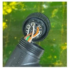
©Screw the screws on both sides of the aviation mouth respectively tight, amphenol aviation head end production is completed.
