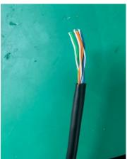
②Peel off about 5mm wire skin of each wire end to expose the copper wire inside, and cut the wire sequence 8 (brown in the picture) about 5mm short.
