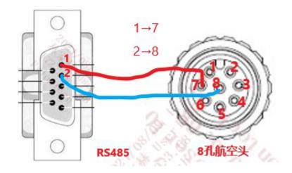
Note that the left and right sides of the gap are port 1 and Port 2 respectively
