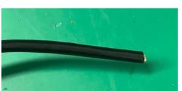
®Peel off the two ends of the wire, about 5mm in length, and cover the copper wire with tin.
