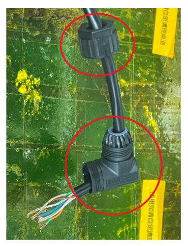
⑤Insert 8 wires into the connecting port of corresponding serial number respectively and lock them with screws. Pay attention to insert part of wire skin into the interface, so that the lock can be tighter.
