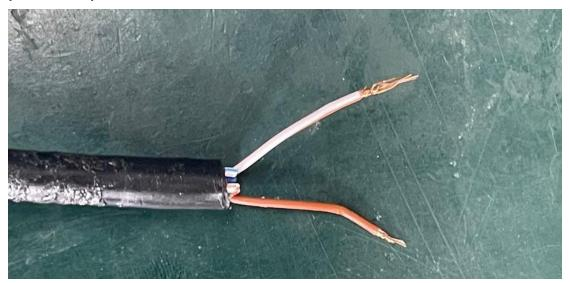
②Put line 7 (white and brown in the picture) into port 1, and line 8 (brown in the picture) into port 2, and screw the connecting port tightly.
