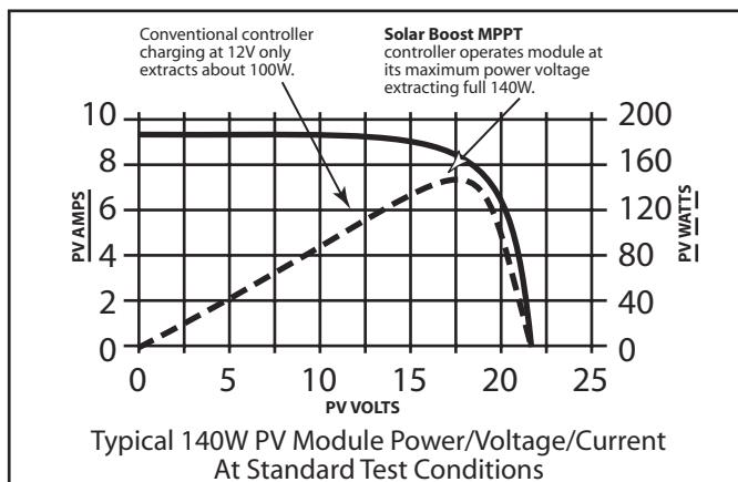
The high efficiency voltage step-down action of the MPPT power converter also allows the efficient use of much higher voltage 60 cell PV modules. Since the voltage delivered by 60 cell modules is much higher than battery voltage charge current increase may approach 200%.
