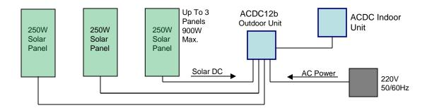
Like all DC-Inverter air conditioners, the ACDC12 compressor runs on DC power converted from AC power. But this special solar air conditioner can also accept DC power directly from solar panels, without needing an inverter, controller, or batteries. The solar DC power directly replaces an equivalent amount of AC power from the power company and can cut daytime energy costs for air conditioning or heating by up to 80-90% or more.
