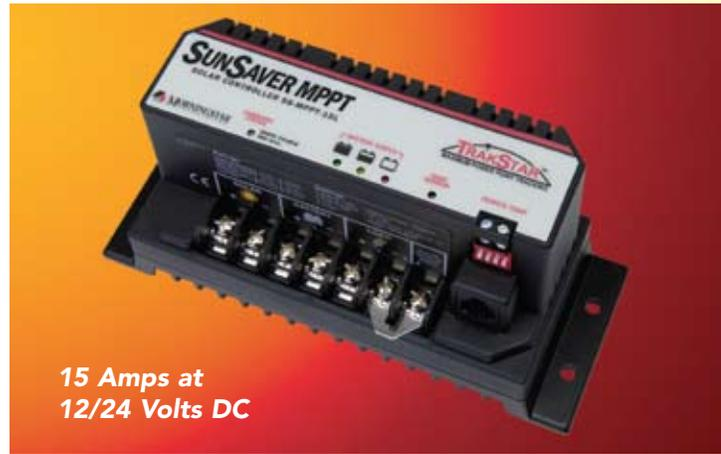
Morningstar's **SunSaver MPPT** solar controller with TrakStar Technology™ is an advanced maximum power point tracking (MPPT) battery charger for off-grid photovoltaic (PV) systems. The controller features a smart tracking algorithm that maximizes the energy harvest from the PV and also provides load control to prevent over discharge of the battery.
