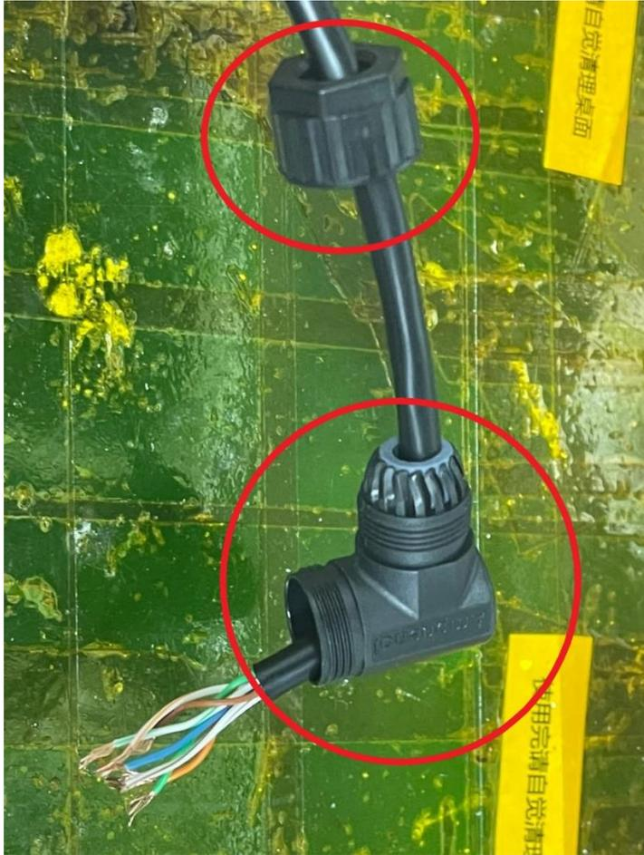
⑤ Insert 8 wires into the connecting port of corresponding serial number respectively and lock them with screws. Pay attention to insert part of wire skin into the interface, so that the lock can be tighter.
