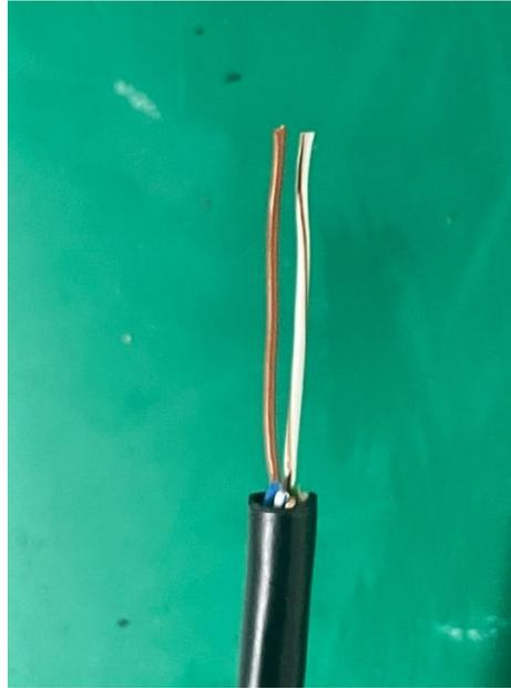
⑧ Peel off the two ends of the wire, about 5mm in length, and cover the copper wire with tin.
