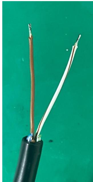
⑨ Cover the two wires with heat shrinkable tubes (the heat
