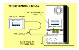
CAT5 port on *TurboCharger*<sup>tm</sup> Network Option Card provides 12 volts to power the Remote Display.
