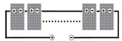
Fig: Series connection for more Voltage
