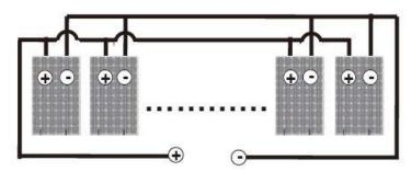
Fig: Parallel connection for more Current
