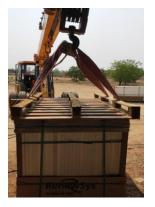
Fig: Packing Box -Adjusting Sling rope for Hoist Handling (Separator - Pallet)
